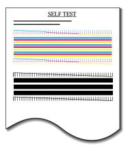
If the diagonal lines are not broken and the bars are clear, the printer mechanism is functioning properly.
